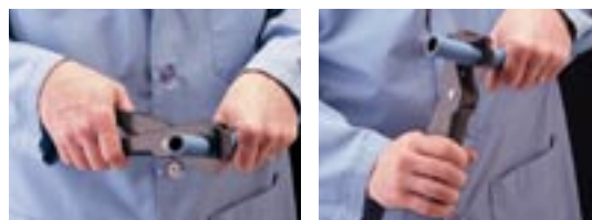
The rotating/rocking technique produces fast easy cuts.
